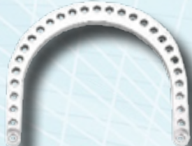
U Ring REF: HOTL03 Size: Ø120, Ø140, Ø150, Ø160 Ø180, Ø200 Material: Aluminum
